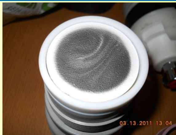
Figure 1: Filter with deposits of Black Carbon
