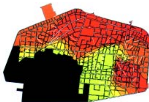
Map 3.1b: Map showing areas that would be inundated in 2050 (high) scenario. That is 1.04m (39.7cm + 64cm*).
