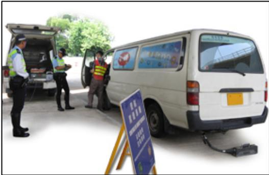
Acceleration Smoke test on the spot using a portable smokemeter. If the vehicle fails to pass the test, the vehicle owner will be fined HK\$1,000 and the vehicle is required to be repaired and retested at one of the Designated Vehicle Test Centres using a lug-down test within 12 working days.
