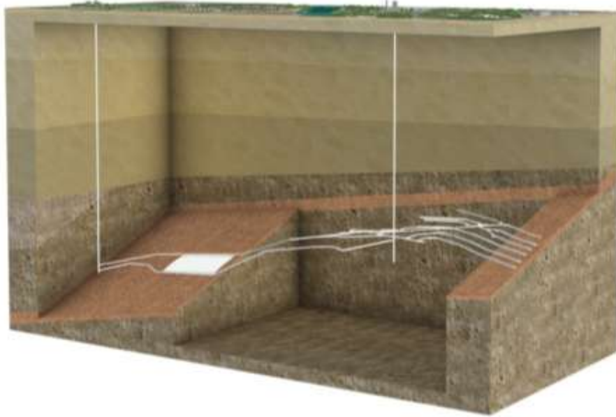
Figure 49 Model of the Konrad site showing the repository horizons and the overburden layers (source: Bundesamt für Strahlenschutz BfS [16]).
