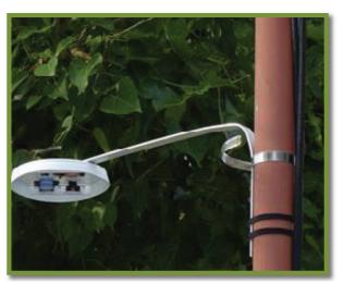
Figure 2. Samplers mounted under rain shield
