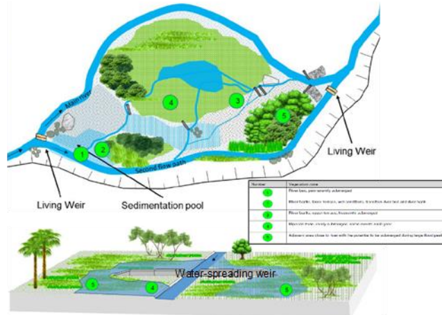
Application of multiple measures in a project site (Living weir, sedimentation pool and plating of local trees)
