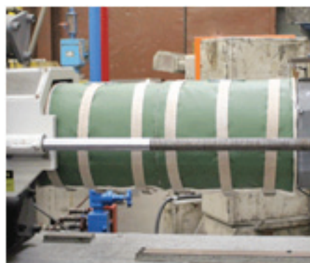
(b) Insulation layer is installed on extruder
